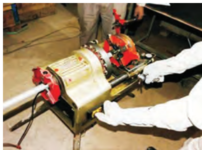
Fig.1.8: Pipe threading using pipe threading machine
