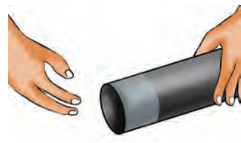
Fig.1.11: Apply the solvent on both the edges
