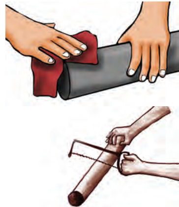
Fig.1.10: Cut and clean the edges of the pipe
