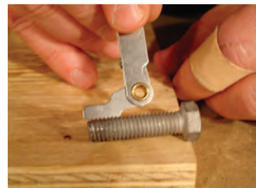
Fig. 1.4: Measuring the thread per inch
