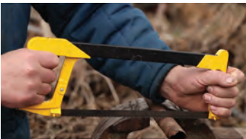
Fig.1.3: Cutting with a hacksaw
