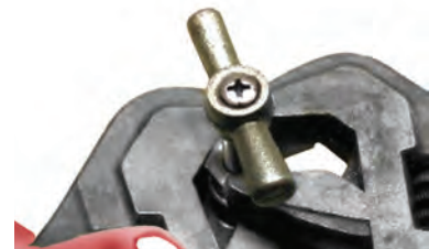
Fig. 5.3: Tightening of a gland nut
