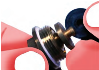
Fig. 5.7: Removing the washer
