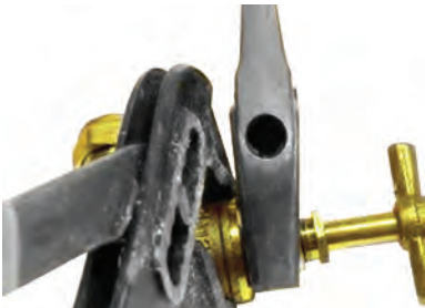
Fig. 5.5: (a) Opening of a large nut
