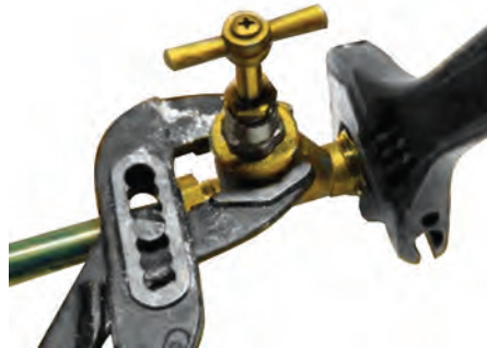
Fig. 5.2: Opening of a compression nut
