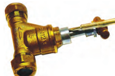
Fig. 5.4: Removing bits from a gland nut
