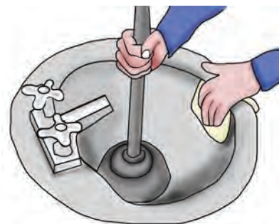
Fig. 5.12: Removing clogs in a washbasin
