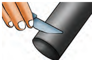
Fig.1.11: Apply the solvent on both the edges
