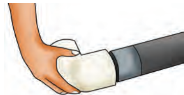
Fig.1.12: Assemble the edges when the cement solvent is wet
