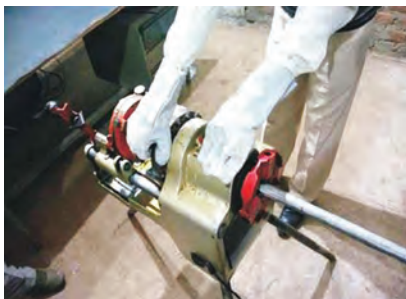
Fig.1.8: Pipe threading using pipe threading machine
