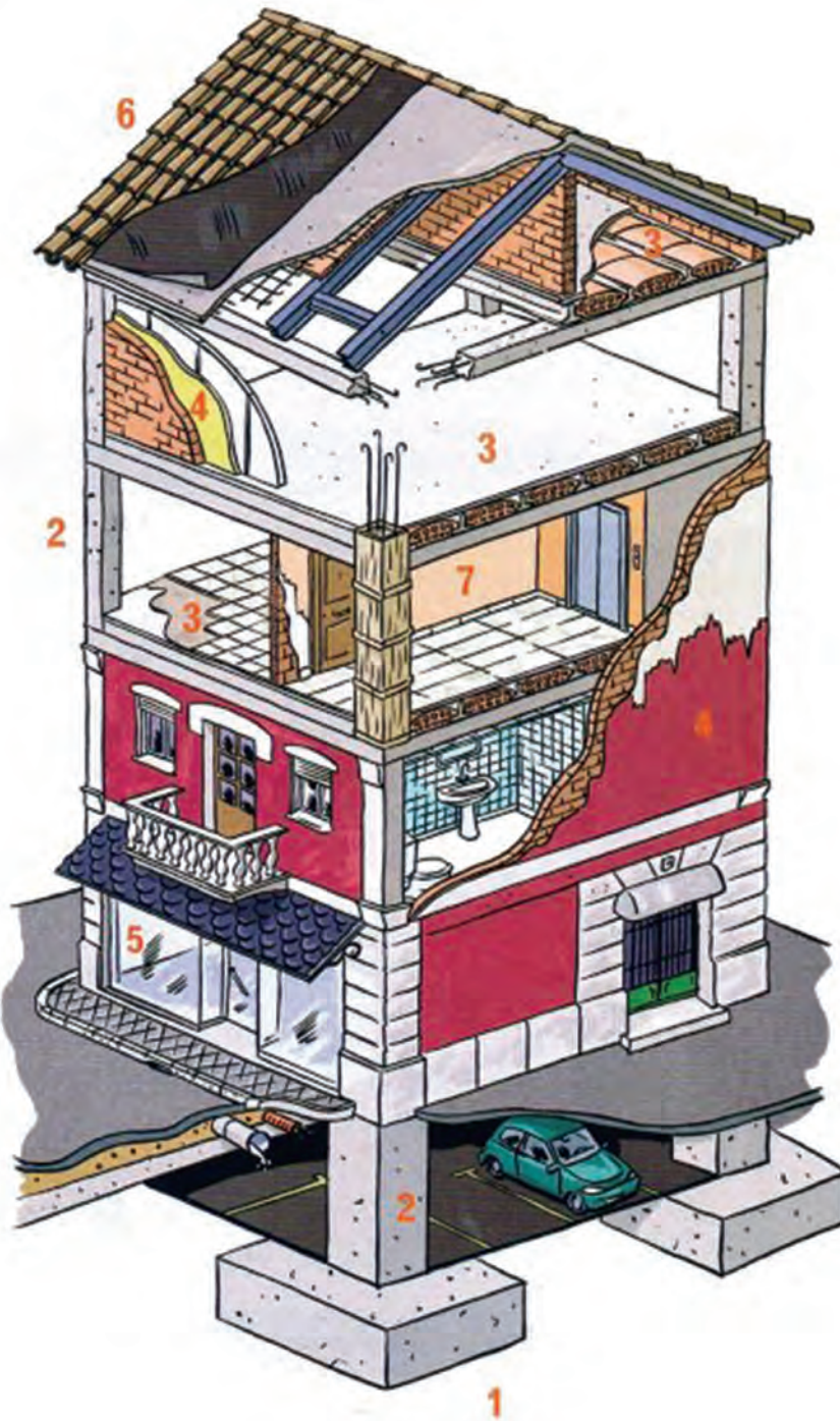
Fig.3.1: Essential elements of a modern building
